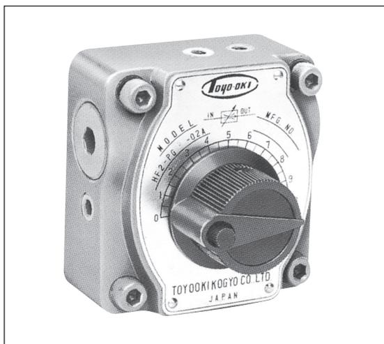
This valve controls flow by changing the cross-sectional area through which fluid flows. Since it incorporates a pressure compensation mechanism, the flow is kept constant even if the pressure varies at the IN and/or OUT port.
