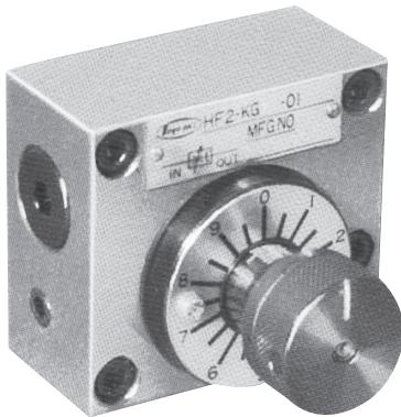
This valve controls flow by changing the cross-sectional area through which fluid flows. Since it incorporates a pressure compensation mechanism and temperature compensation mechanism, the controlled flow is kept constant regardless of the pressure variation at the IN and/or OUT port and the viscosity variation due to temperature change.
