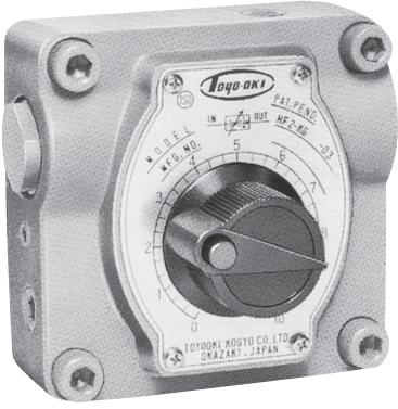
This valve controls flow by changing the cross-sectional area through which fluid flows. Since it incorporates pressure compensation mechanism and temperature compensation mechanism, the flow is kept constant regardless of the pressure variation at the IN and/or OUT port and the viscosity variation due to temperature change.
