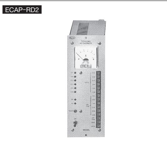
This control amplifier is constructed compactly by adopting a switching power supply and can operate with a wide range of power supplies (85 to 250 VAC (50/60 Hz) and 110 to 250 VDC).
